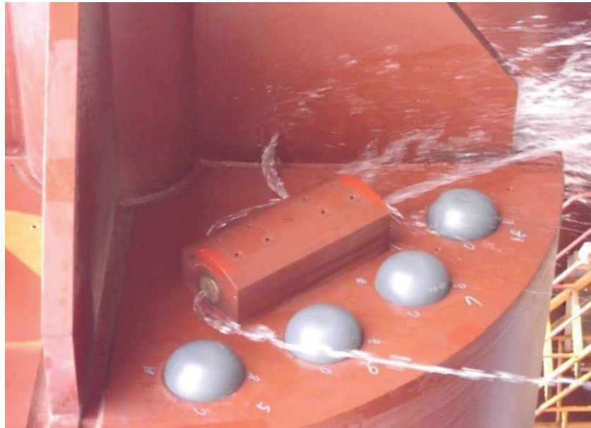
Figure 6-13 Jetting Operation from Nozzle Block (Without Spudcan)
